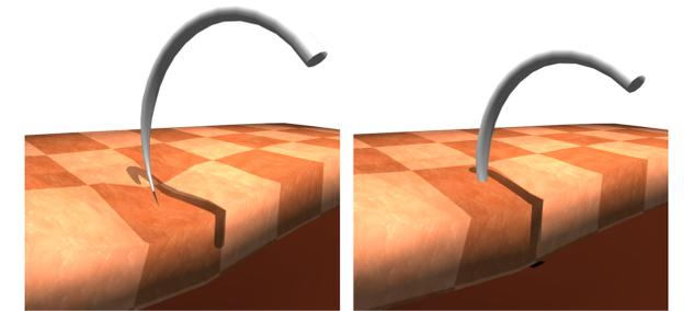
Contact between the needle tip and the tissue is modeled differently: if the interaction force reaches a puncturing force threshold, the needle starts penetrating the soft tissue.
